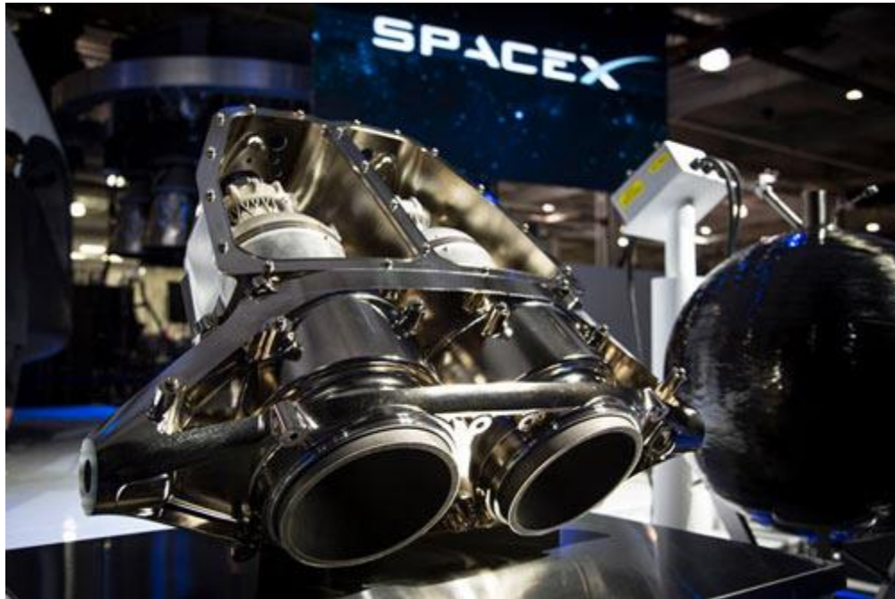
Figure 7 3D printed rocket engine by SpaceX [6].
