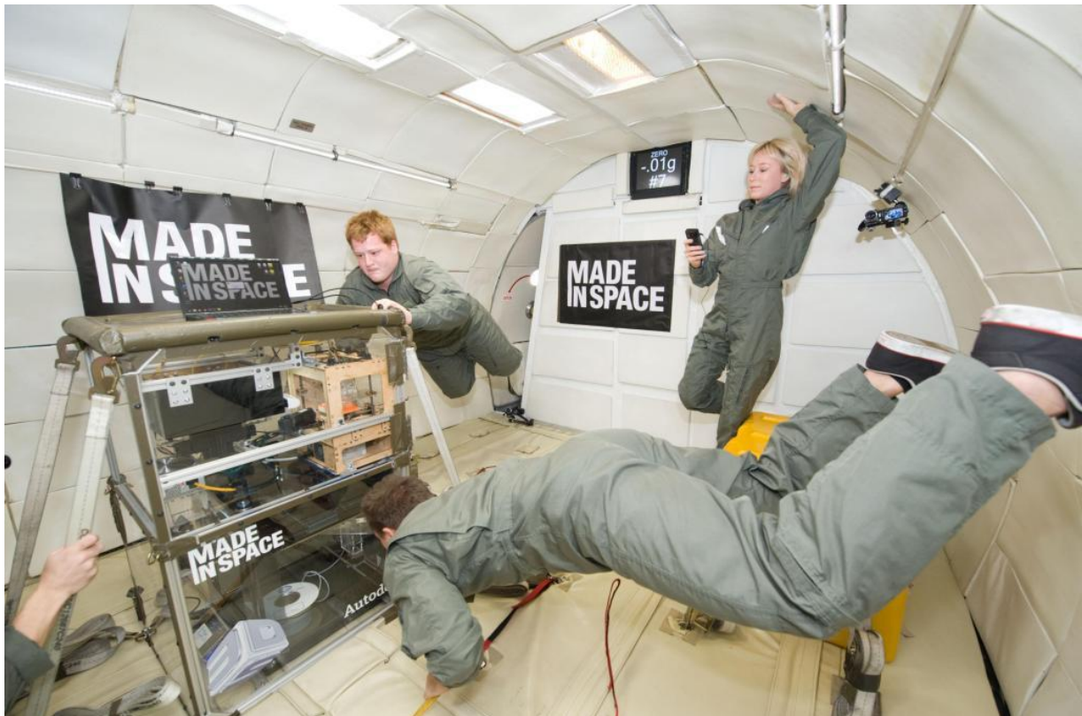
Figure 8 A 3D printer passing microgravity flight tests [14].
