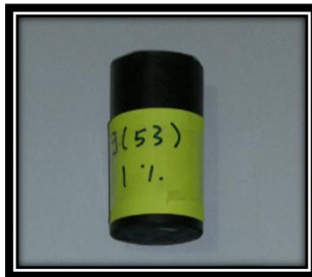
Figure 2 Sample of Compression Test
